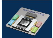
Process Data Move Data Store Data The Intel® Agilex™ FPGA F-Series, I-Series, and M-Series family brings together the power of Intel's 10 nm SuperFin and Intel 7 technology, heterogeneous system-in-package (SiP) integration with Intel's proprietary Embedded Multi-Die Interconnect Bridge (EMIB), and an innovative chiplet-based architecture to deliver customized connectivity and acceleration for a variety of applications.
